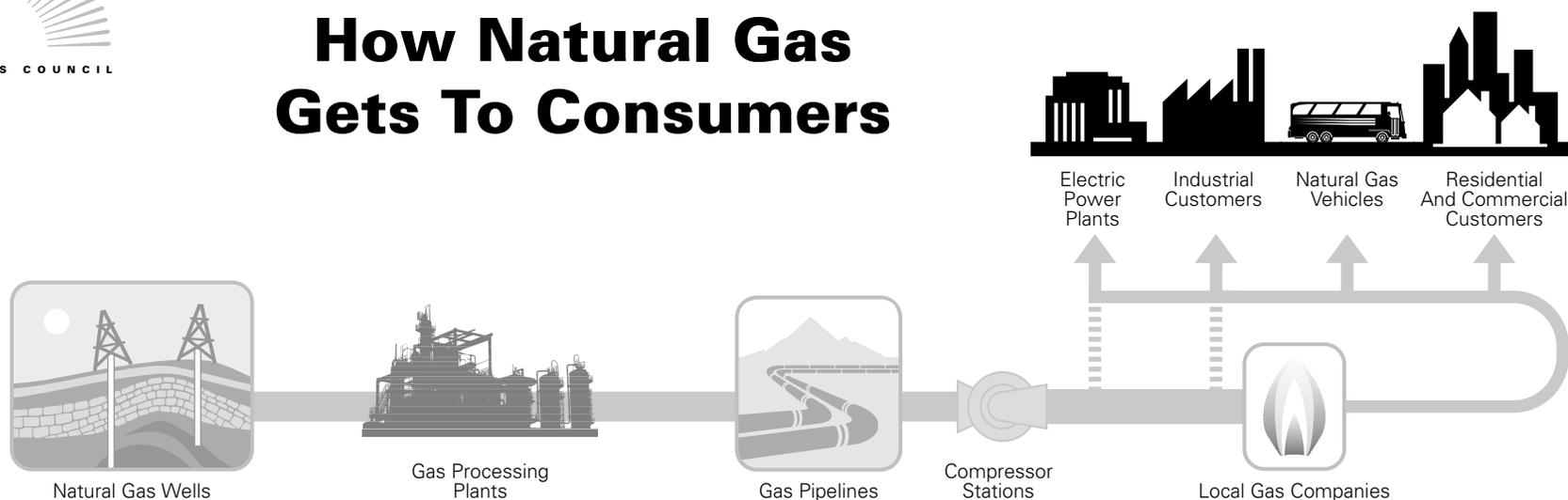
Natural gas is a naturally occurring hydrocarbon that consists mostly of methane. It is usually found in underground formations of porous rock, and found either alone or in association with oil. During the **production process**, wells are drilled into the porous rock and pipes are used to bring the natural gas to the surface. In most wells, the pressure of the natural gas is enough to force it to the surface and into the gathering lines.
